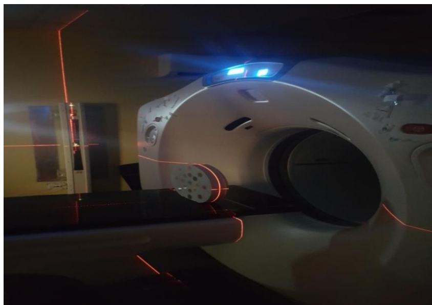
Figure 2: Set-up of the phantom using external lasers.
