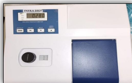
Figure 2: Photographic view of optical density of the growth seen in test tubes will be measured in spectrophotometer at 600nm.
