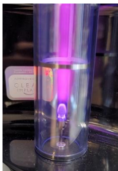
Figure 7: Visible UV light radiation on the titanium fixture with the Actilink Reborn by Plasmapp.
