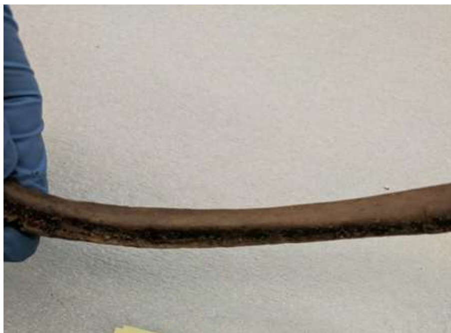
Figure 3: Control without Notching Present.
