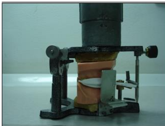
Figure 2: Closed semi-adjustable articulator with mounted models, dual-arch tray, vertical tray positioner, tray clamping jig and 1.5 kg weight on top.
