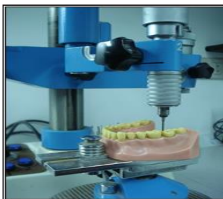
Figure 1: Cutting bur orientation parallel to the long axis of the prepared model.
